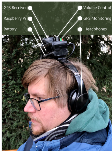
Figure 5: Components of the sonification device
