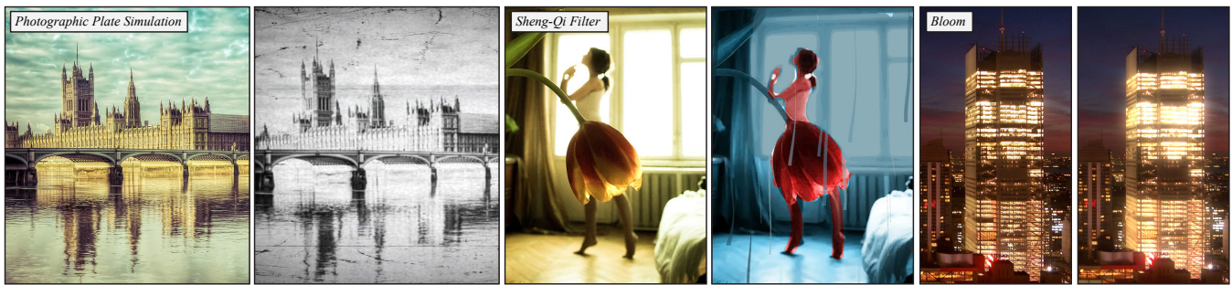
Figure 8: Additional effects implemented by our undergraduate students as part of a seminal project, using the proposed framework for development: (left) photographic plate simulation based on unsharp masking, grayscale rendering and noise, (middle) simulation of the Sheng Qi painting style by rendering with spot colors and visualizing paint drops, (right) bloom effect based on lightening image regions.
