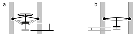
Figure 23: (a) The spring we use in our bit cells is longer and thus weaker than (b) conventional bistable springs. Or, for the same force, our cells produce more stroke length.
