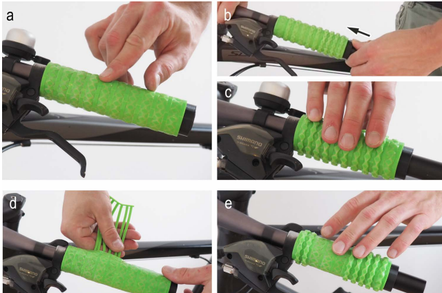
Figure 6: (a) Designers fabricate one single bicycle grip that they (b) actuate continuously to different levels, (c) to feel the tactile qualities during rapid prototyping. (d) By inserting spacers after fabrication that (e) deactivates selected rows allows them to further investigate the grip’s ergonomics.
