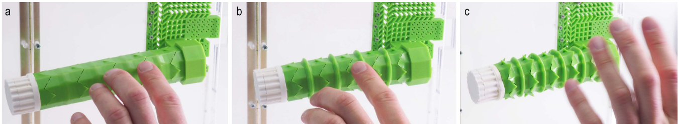
Figure 1: When an external force is applied, metamaterial textures undergo a controlled transformation. This door handle, for example, transforms (a) from flat (b) to rippled (c) to spiky, allowing the person behind the door to set a tactile message with three levels of enter/busy/do not enter messages for visually impaired or sighted users trying to enter.
