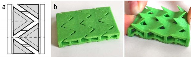
Figure 14: (a) Leaving gaps between the members of the cell top (b) allows for creating spikey textures.
