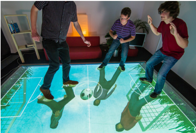
Figure 8: GravitySpace allows for interaction with virtual objects as leg movement is tracked above the floor by analyzing the center of pressure of the other foot.
