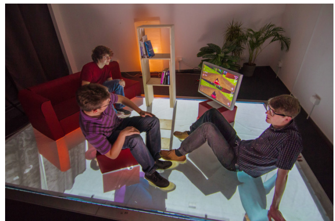
Figure 7: Daniel and René are controlling a video game by simply leaning over, tracked by observing varying centers of pressure. GravitySpace also detects that Andreas sits down, based on the body parts in contact with the floor.
