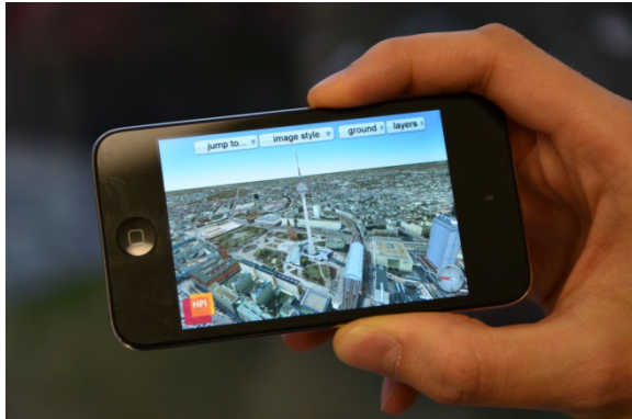
Figure 1: 3D client for exploring the 3D city model of Berlin, running on an iPod.
