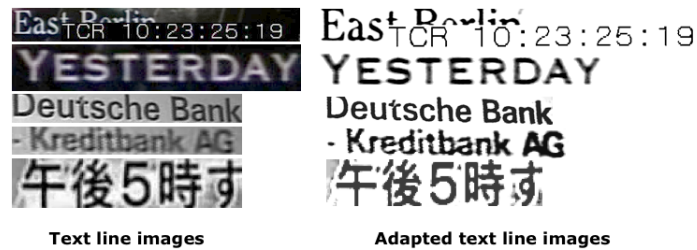
Figure 12: Exemplary resulting images of dynamic contrast/brightness adaption. Contrary to the originals, the revised images are suitable for being processed by OCR engines, as the background has been removed.
