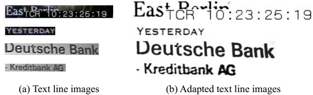
Figure 8. Example resulting images of dynamic contrast/brightness adaptation. Contrary to the originals, the revised images are suitable for being processed by OCR engines, as the background has been removed.
