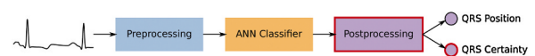
Fig. 7. The change this work proposes to the architecture shown in Fig. 5 (marked with a red frame). We propose generating not only QRS positions but also a certainty score for each position. Therefore, the postprocessing part needs to be changed.
