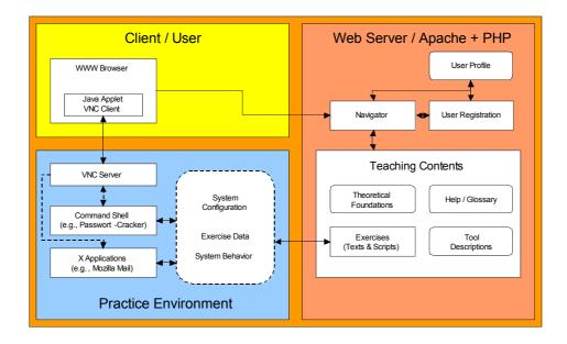
Figure 1: TELE-LAB IT-SECURITY system architecture
