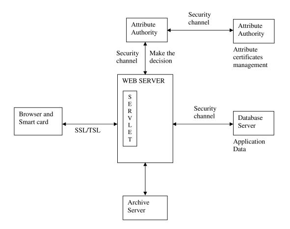
Figure 3. HARP Cross Security Platform Architecture
