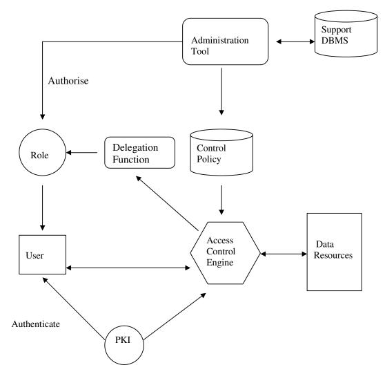
Figure 4. Overview of the access control system
