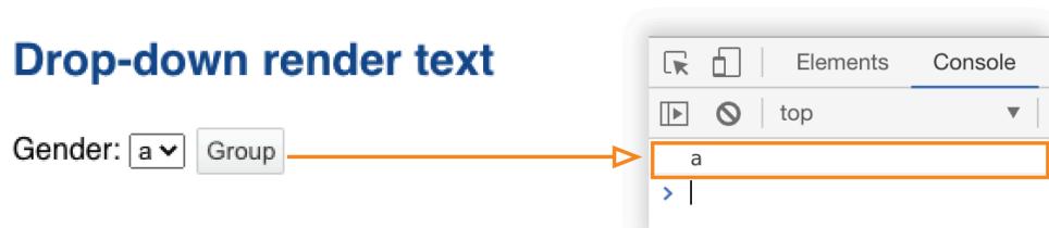
Figure 4.7: Rendered markdown with executed scripts and native HTML elements embedded
