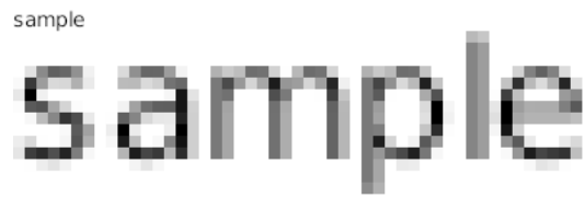
Figure 4.12: The picture shows ‘sample’ rendered with antialiasing. The text was rendered at a smaller size and then scaled up to show details. The result is grey-scale, the hue depending on how the curves of the glyph pass through the pixel. At normal size the text is a bit blurry because of the many light tones. (Source: https://upload.wikimedia.org/wikipedia/commons/0/09/Rasterization-antialiasing-without-hinting-2.png , visited on 2017-07-27)
