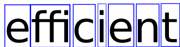
Figure 4.15: The picture shows the text ‘efficient’. All separate glyphs are encased by rectangles to show which glyph objects would be needed to create the text. Noticeable ‘ffi’ is one glyph because it is a ligature.
