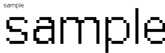
Figure 4.11: The picture shows ‘sample’ rendered very basic without antialiasing. The text was rendered at a smaller size and then scaled up to show details. All pixels are completely black or white which leads to sharp edges. (Source: https://upload.wikimedia.org/wikipedia/commons/8/8c/Rasterization-simple.png , visited on 2017-07-27)
