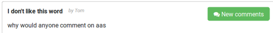
Figure 2.10: The ThreadPreviewWidget gives a concise overview of a single thread. When there have been new comments since a user's last visit, the button on the right indicates this by turning green.
