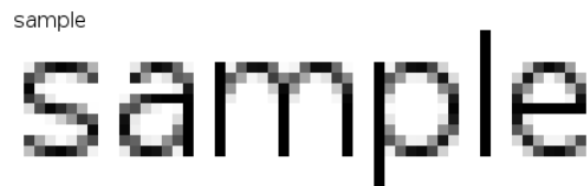
Figure 4.13: The picture shows ‘sample’ rendered with antialiasing and hinting. The text was rendered at a smaller size and then scaled up to show details. The hinting helps determining which pixels should be darker to create a less blurry result. (Source: https://upload.wikimedia.org/wikipedia/en/e/ec/Rasterization-antialiasing.png , visited on 2017-07-27)
