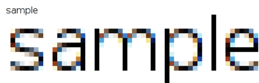
Figure 4.14: The picture shows ‘sample’ rendered with subpixel rendering. The text was rendered at a smaller size and then scaled up to show details. A pixel contains three subpixels in different colours. Using these can create a clearer image. This technique is dependent on the displaying hardware. (Source: https://upload.wikimedia.org/wikipedia/commons/0/0b/Rasterization-subpixel-RGB.png , visited on 2017-07-27)
