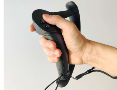
Figure 2. Picture of the Valve Index controller. The index finger is placed at the trigger button. Middle, ring, and little finger determine the strength of the grip input. Using their thumb, users can control a touchpad, a thumbstick, and several buttons.
