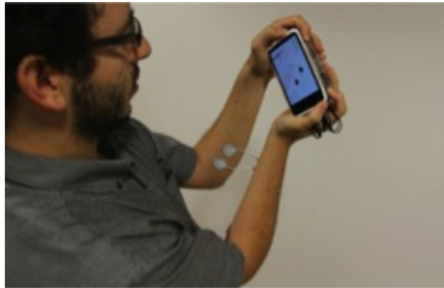
Figure 1: We developed a mobile force feedback device that electrically stimulates the user's muscles, instead of using mechanical actuators.
