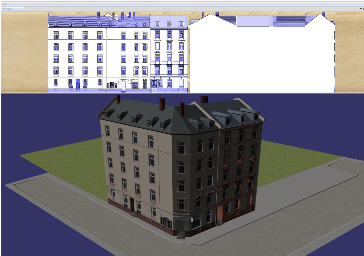
Figure 7: Screenshot of the prototype. The prototype consists of two separated view-ports: The 2D building panorama (top) and the 3D perspective view (bottom). Based on the use-case, the 2D building panorama serves as detail or overview visualization for the 3D perspective view.
