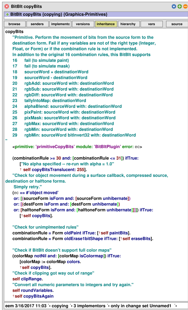
Figure 5: On failure, adjust BitBlit’s object state and retry the primitive.
