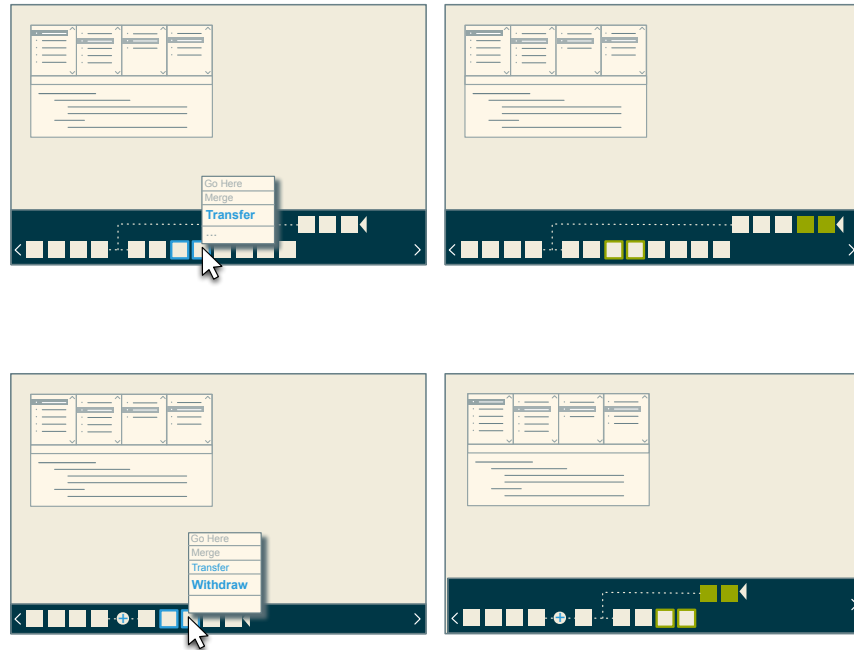
Figure 21: Top row: Selecting two changes and re-applying them to the currently active version (triangle). Bottom row: Withdrawing two changes, which results in re-applying subsequent changes to the change before the selection
