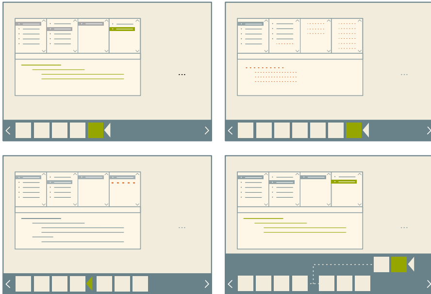
Figure 9: (From top left to top right) A programmer modifies source code, which implicitly creates items in the version bar. The filled triangle marks the current position in the history - the version that is currently active. When a programmer goes back to a previous version (bottom left), and then continues working, the new changes will appear on a new branch that is implicitly created (bottom right).
